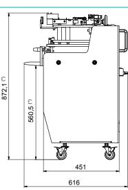
(\*) The working height depends on the installation.
